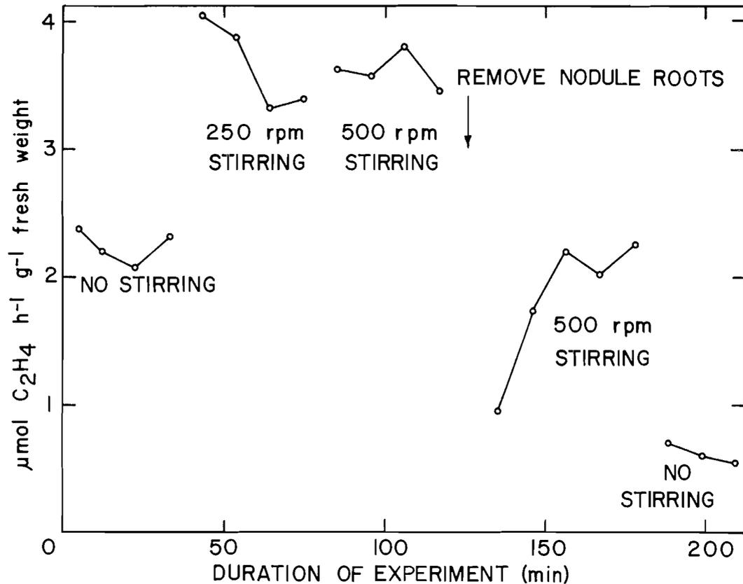
FIG. 4. Effect of stirring rate and nodule root removal on acetylene reduction by whole plants. The shoots were in air and the roots were in a nutrient solution equilibrated with 0.05 atm  $pO_2$  and 0.1 atm  $pC_2H_2$ . 1 atm = 101.325 kPa.
