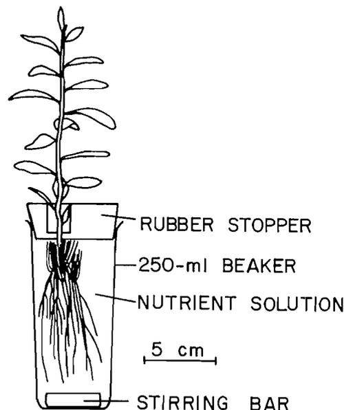
FIG. 1. Apparatus for measuring acetylene reduction with roots in a nutrient solution.
