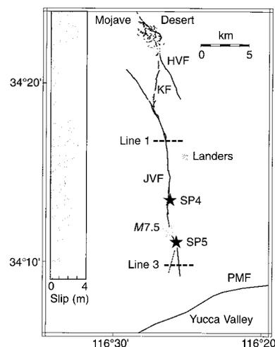
**Fig. 1.** Map of the study region showing locations of two seismic arrays at line 1 and line 3 and two explosions SP4 and SP5 in the fault zone of the 1992 Landers, California, earthquake. Only the southern half of the Landers rupture lies within this map, and the dextral surface-fault slip profile is shown (inset) to the left of the map (12). JVF, Johnson Valley fault; KF, Kickapoo fault; HVF, Homestead Valley fault; and PMF, Pinto Mountain fault.
