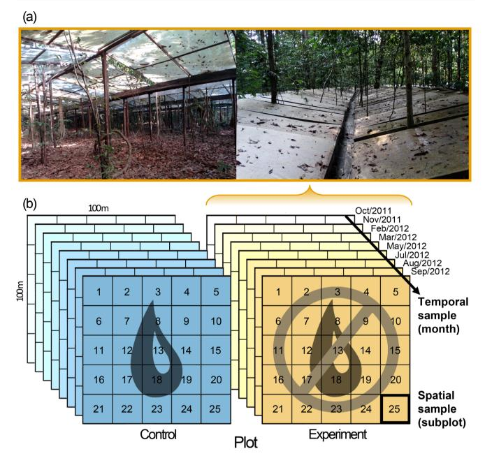
**Fig. 1 a** Photos obtained from below (left) and above (right) of the plastic panels that exclude rainwater at the experimental plot. **b** Experimental design for both plots (control and experimental), illustrating the temporal (months) and space (subplots) samples for col-
