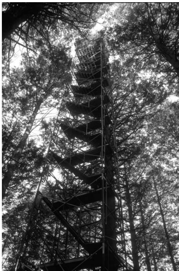
PLATE 1. Eddy covariance tower in a hemlock stand at the Harvard Forest. Photo credit: J. Hadley.
