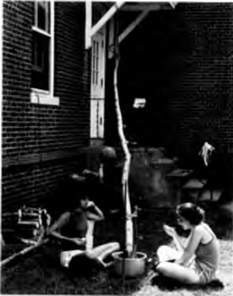
*Calculating vessel length distribution in a stem of white ash by measuring the rate of air flow through successively shorter stem segments at given pressure gradients. From left to right: Monica Mattmuller, Martin Zimmermann and Liz Markell. (Photograph by Bill Ormerod)*
