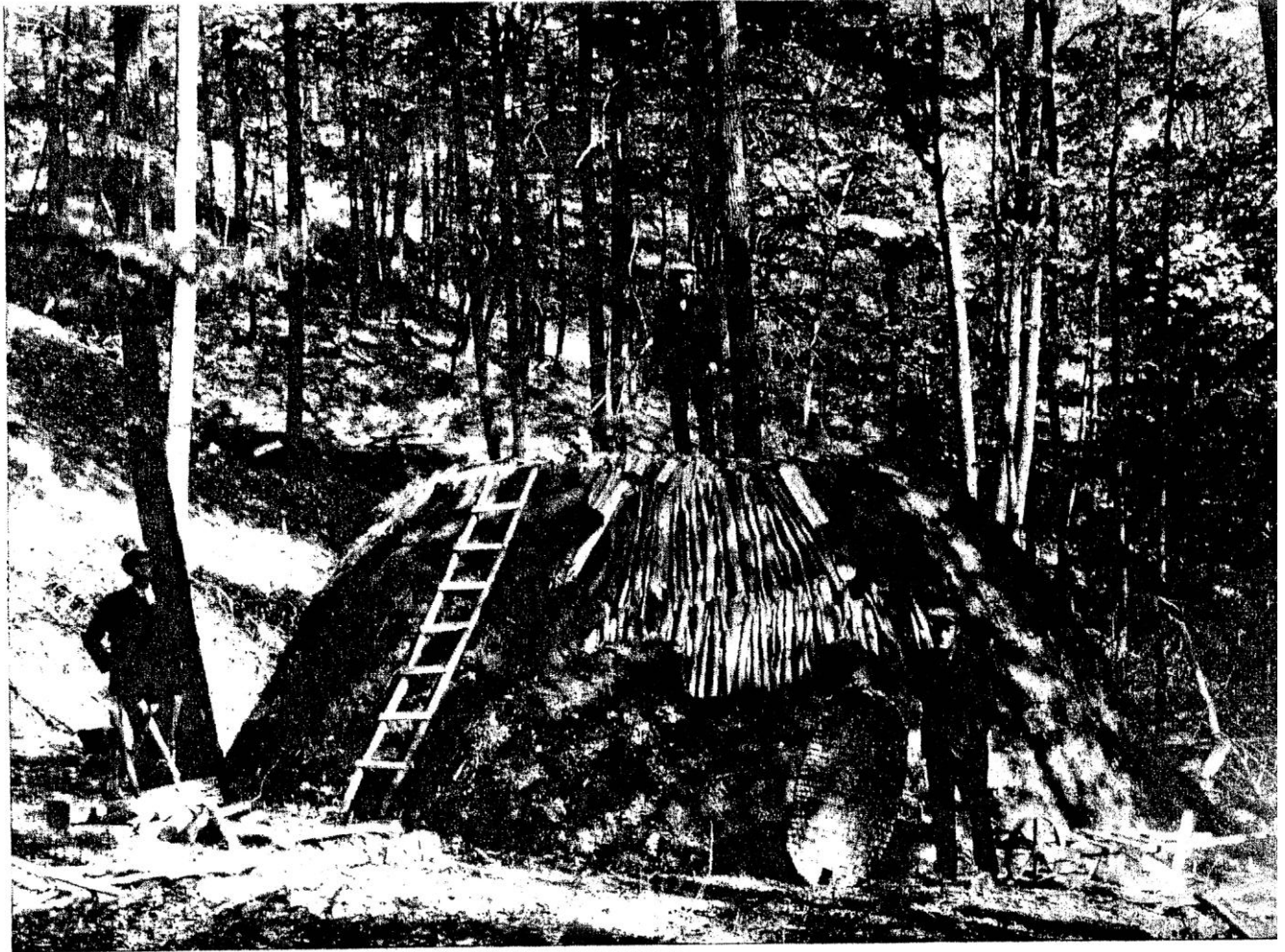
PLATE I. OPEN-PIT PROCESS, SHOWING THE STACK NEARLY COVERED WITH THE "FLOATS
