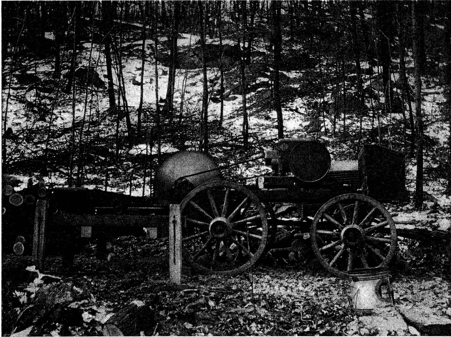
PLATE V. SIDE VIEW, CLOSE-UP OF WOODSAW. NOTE STURDY TRACK CARRYING SLIDING TABLE; SLOTTED, EXTENSIBLE LEGS, AND GENERAL COMPACTNESS, ESPECIALLY OF THE 5 HP I.H. ENGINE.
