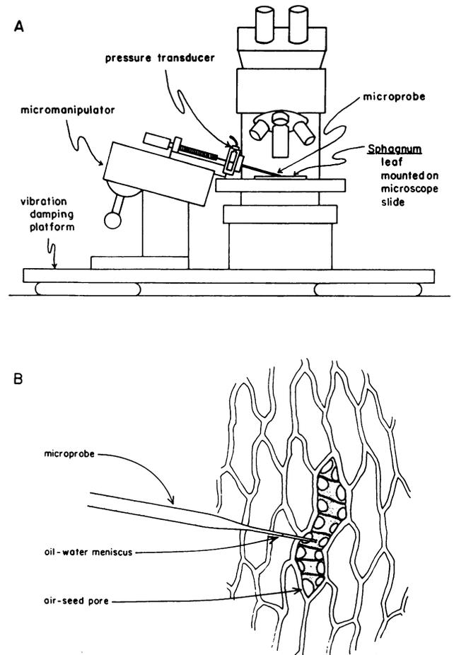
FIG. 3. Pressure microprobe setup. A, Microprobe apparatus; B, microprobe inserted into hyalocyst.
