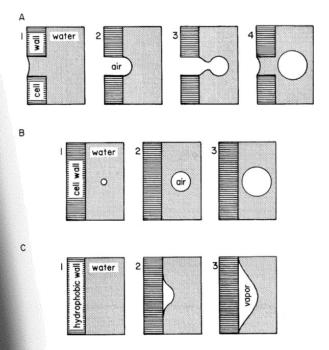
Fig. 1.2. Continuity among processes that initiate embolism. It may be difficult to distinguish between a free-floating bubble and a bubble that is trapped in a crack in the cell wall, as in A; between a bubble in contact with external air via a crack in the cell wall and an entrapped bubble which has no contact with external air, as in B; and between separation at a hydrophobic surface and expansion of a bubble trapped at a hydrophobic surface, as in C.
