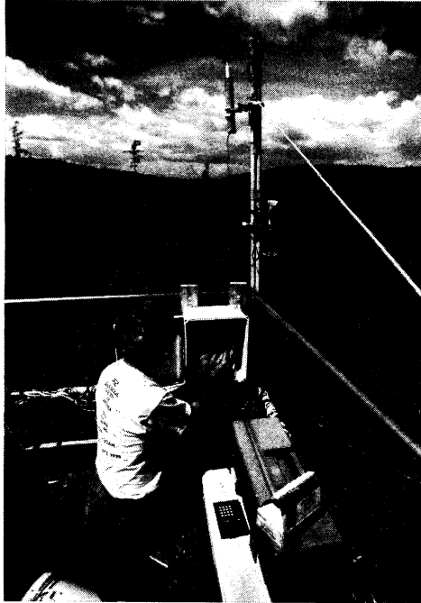
Figure 17.3. An eddy flux system that records exchanges of \text{CO}_2 and other material between the forest and the atmosphere. One of three such systems in operation at the Harvard Forest, this equipment is situated above an old-growth hemlock forest in the center of the Prospect Hill tract. Results are compared with detailed physiological and ecosystem results and are being used to develop a simple model of forest ecosystem function. The canopy walk-up tower used for this system also provides access to leaves, branches, and boles of the tree for detailed physiological measurements. Photograph by J. Gipe.
