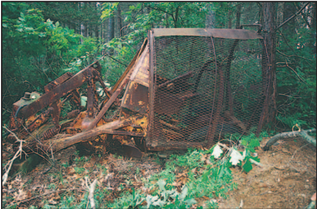
Figure 18. Equipment used for machine-planting conifer seedlings in the 1960s in MFCSF. Top: plow pushed in front of large tractor. Bottom: planting cage with disc and small plow.
