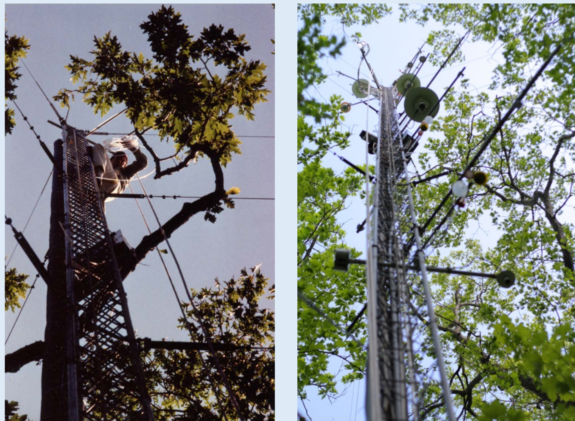
Then and now: photos of Bill setting up the eddy covariance tower in 1991 (left), and what the tower looks like now (right).
