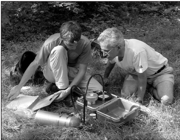
Chris Graham and Julian Hadley using a Scholander pressure chamber to measure leaf water potentials after a carbon dioxide exchange measurement
