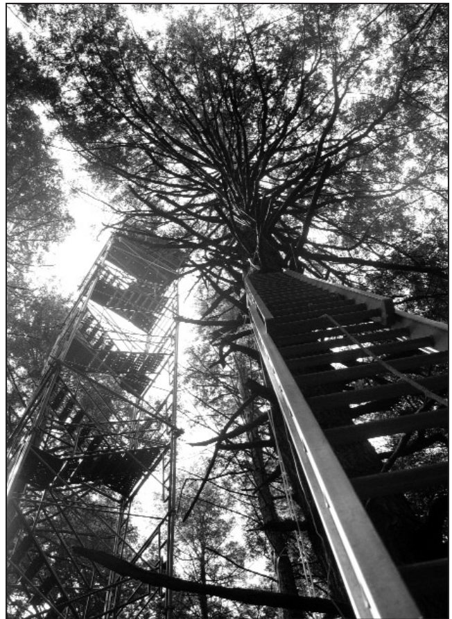
Walk-up tower for sampling gas exchange in the Prospect Hill hemlock stand
